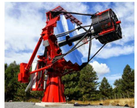
to reflect the Cherenkov light to a high-speed camera that can digitize and record the image of the shower. Above, an SST prototype in Italy.
