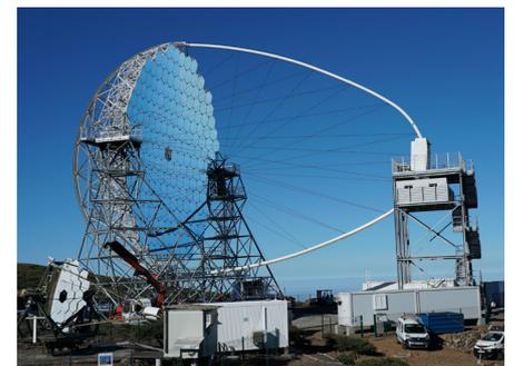
respectively) to reflect the Cherenkov light to a high-speed camera that can digitize and record the image of the shower. Above, the LST prototype on La Palma. Credit: Iván Jiménez, IAC
